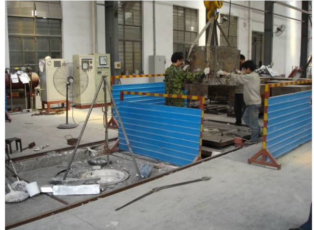
Low Pressure Casting Hardsand Moulds at Wuxi Aluminium Technology Co Ltd
